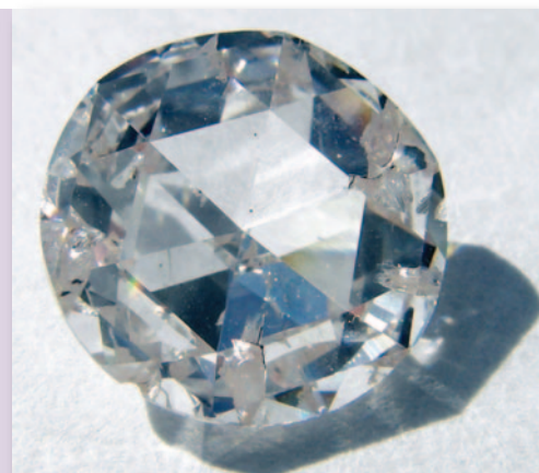
This rose-cut synthetic diamond was created using the CVD process. Wikimedia/Steve Jurvetson
