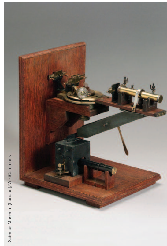
William Henry Bragg's X-ray spectrometer as used by him and his son William Lawrence Bragg to investigate the structure of crystals
