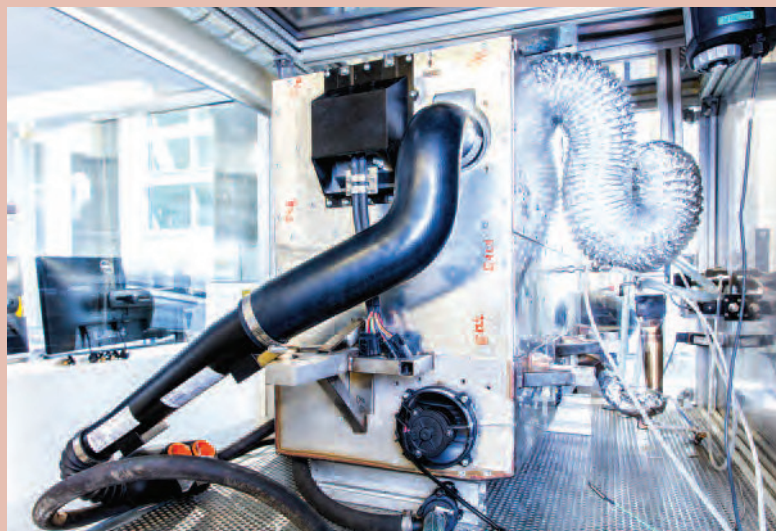
Nissan's SOFC system test bench. The system generates electricity from ethanol and air to charge the battery.
