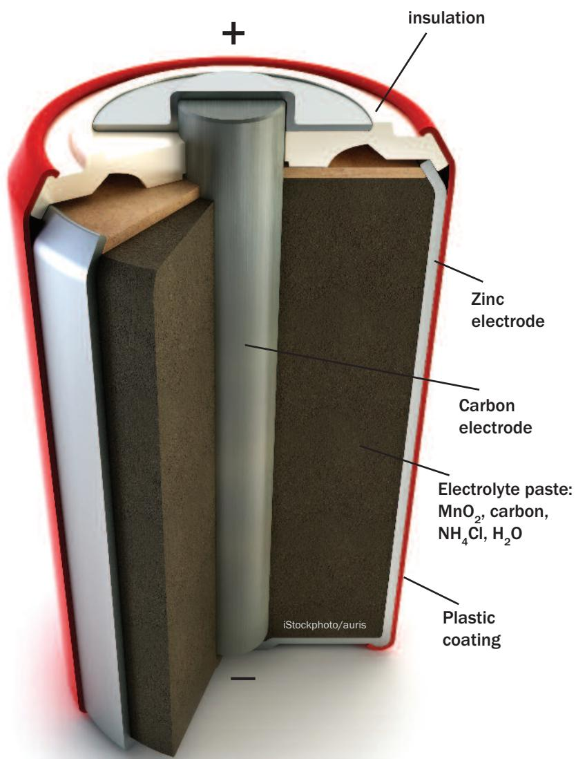
Cutaway diagram of a type of dry cell battery. Dry cell batteries are named for their electrolyte (conducting medium), which is a paste rather than a solution. Alkaline, lithium, nickel–metal hydride and silver oxide ('button') cells are all types of dry cell.
