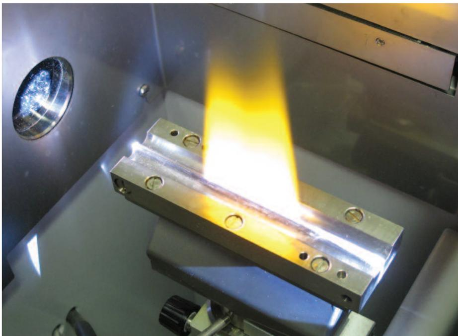
The high-intensity continuous spectrum light of the ContrAA's xenon short-arc lamp is visible in the window and along the length of the burner.
